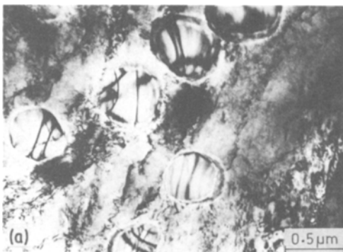
Figure 6 (a) Coarsening of the individual precipitates on ageing at 703 K for 10 min. (b) Coalescence of the \gamma phase particles during ageing at 653 K for 90 min.
